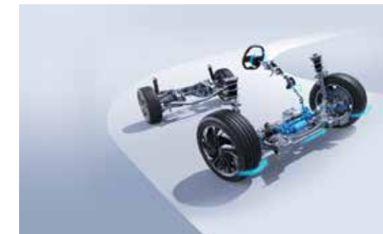
ACCURATE STEERING The new DUAL PINION steering system provides precise cornering, as you wish.
